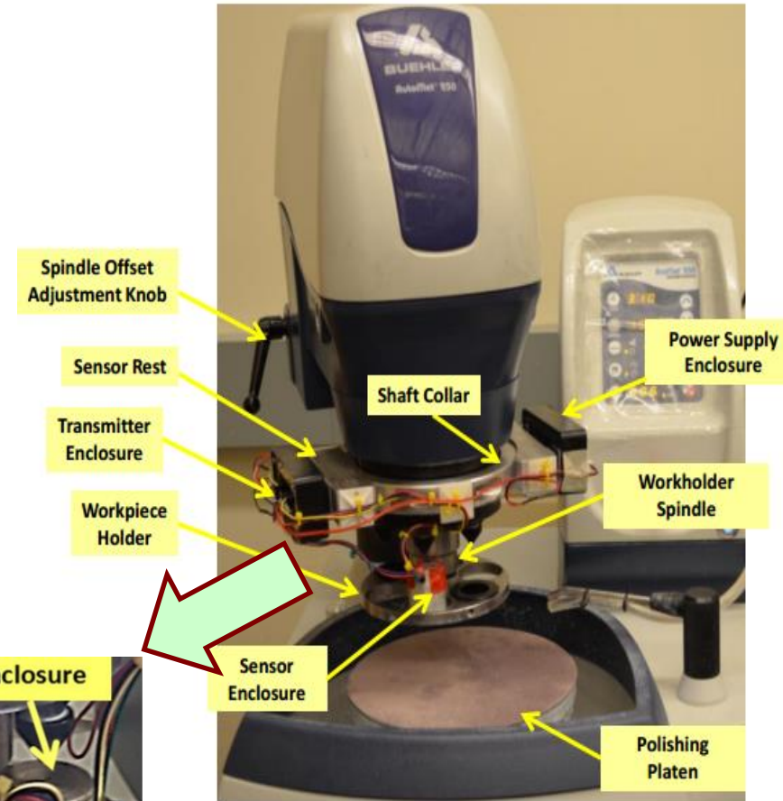
Buehler (model Automet ® 250) with 3-axis accelerometer
